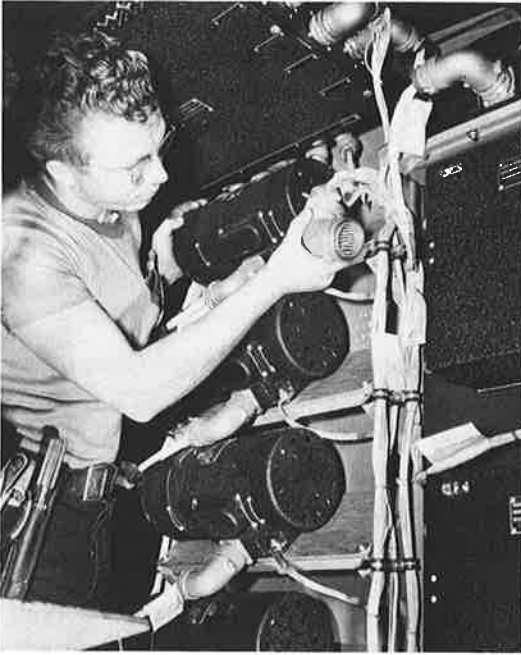
Amphenol connectors and cable being installed in a Boeing B-29 Superfortress
